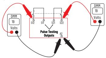
3. If a significant difference in voltage levels exists, see <u>Capacitance Effect on page 61</u> and <u>Long Wire - Resistance Effect on page 62</u>.
