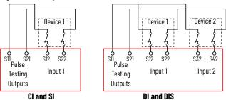
Figure 9 shows the typical connections for devices with 1 N.C. mechanical contact. One side of the contact is connected to a pulse-testing output S11. The other side is connected to two input terminals. The CI and SI safety relays only have one set of input terminals. The DI and DIS safety relays have two sets of input terminals. The DI and DIS safety relays can operate with only one device that is connected or with devices that are connected to both inputs.
