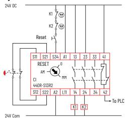
Figure 44 on page 46 shows a CI safety relay monitoring a safety light curtain with two OSSD outputs. The CI safety relay is set to automatic/manual reset (AM). The auxiliary signal (terminals 41/41) informs the PLC that the safety system is off or on. The CI safety relay outputs connect to AC voltage loads. When the CI safety relay is on, the PLC can then turn on the K1 and K2 contactors.
