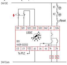
The DIS safety relay monitors two devices with OSSD outputs in Figure 48. The DIS safety relay logic setting is 6: (IN1 AND IN2) OR L12 with automatic reset. The output terminals 34 and 44 are designed to tolerate higher capacitance loads (but lower resistive load) as compared to terminals 14 and 24.
