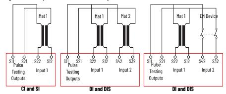
Because the safety mats are parallel plates, they have a significant capacitive effect. The larger the safety mat, the more capacitance. If the capacitance is too large, the safety relay does not function properly. See <u>Capacitance Effect on page 61</u> for further information.
