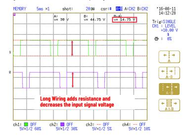
Figure 69 - Resistance Effect on Input Signal
