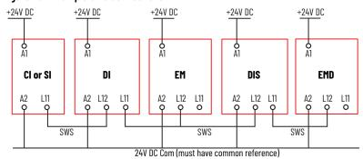
For long wire runs of the SWS signal, a shielded cable can be necessary to help prevent nuisance faults from electromagnetic and motor noise.
