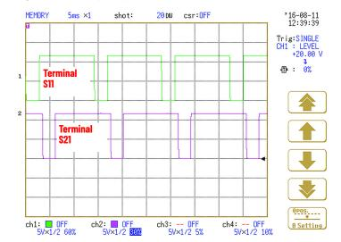
Figure 66 - CI Safety Relay Pulse Test Waveforms
