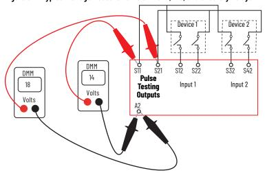
2. Check the voltage at each of the inputs with the device contacts closed. The values must be very close to the values measured at terminals S11 and S21.
