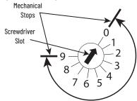
**IMPORTANT** Adjust the switches gently and do not turn past the mechanical stops.
