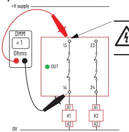
**SHOCK HAZARD:** Remove the power connections to terminal 13 before measuring the contact resistance.
